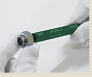
First, the GO side should thread into hole without
